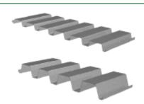
Use of 1.5B, 22 or 20 gage deck is very common. The 1.5 indicates the rib height of the deck.
